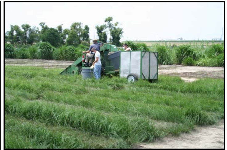
The warm season perennial grass variety trials in Tifton (left) and the flail-type plot harvester used to measure forage yield.
